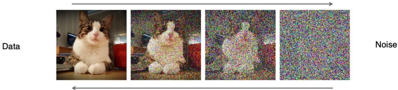
Train a neural network to iteratively transform a **noisy** sample to **clean** or real data.
